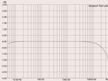
**Graph 4.** Frequency response of line input at an output of 1-watt into an 8-ohm non-inductive load (black trace) and into a combination resistive/inductive/capacitive load representative of a typical two-way loudspeaker system (red trace).
