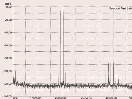
**Graph 3.** Intermodulation distortion (CCIF-IMD) using test signals at 19kHz and 20kHz, at an output of 1-watt into an 8-ohm non-inductive load, referenced to 0dB.
