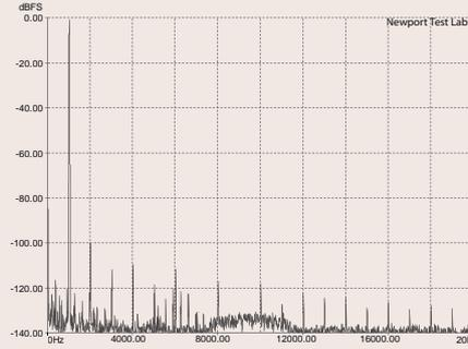
**Graph 2.** Total harmonic distortion (THD) at 1kHz at rated output (100 watts) into an 8-ohm non-inductive load, referenced to 0dB.
