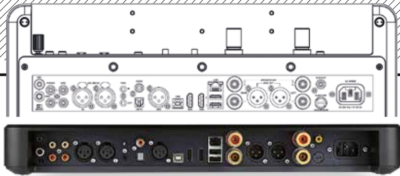
ABOVE: From left to right – room EQ mic socket; phono, RCA and XLR line inputs; trigger plus coax/optical S/PDIF, AES/EBU, USB, I 2 S (two on HDMI) and LAN inputs; 4mm speaker cable binding posts with balanced preamp outs and a sub out on RCA
