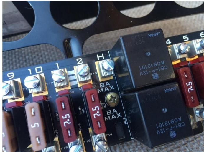
Fitting the extra headlamp feed can help to spread the current load on cars with additional equipment, even though standard headlamps are fitted.
