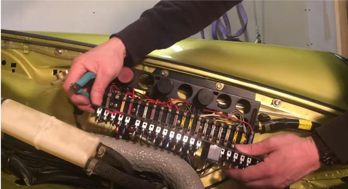
8. Again, starting at the left hand end, transfer each top row wire across to the new panel. These are replicated on PCB of the new panel so do not need to be fitted. This time, you will be able to remove the three original blocks as you go along for improved access.
