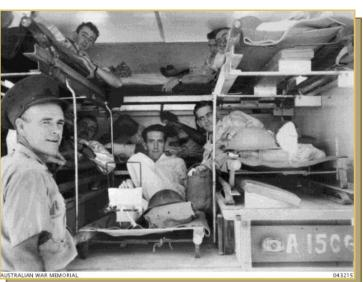
Like the Indian Pattern Ambulance, the Austins were equipped with racking for four stretchers, or could be reconfigured for seated casualties. AWM P01373.005.
