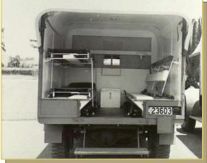
The interior of an Indian Pattern ambulance, showing the two-tiered stretcher rack erected on the left, while the rack on the right side has been collapsed to accommodate seated patients. Registration C-23602 was a 1941 model Chevrolet 30cwt assembled at GM-H's Pagewood plant in Sydney. The ambulance body was manufactured at Woodville, South Australia. AWM069592.
