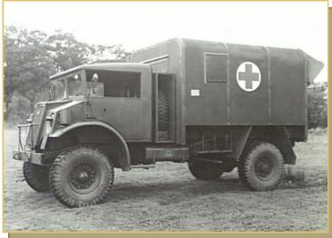
A Chevrolet C30 based 'Truck, 3 ton, Ambulance (Aust)', this one featuring a timber spare tyre stowage box, and a POW rack under the bodywork. AWM 069720.
