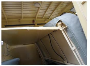
This photo shows the wooden lathes that form the roof structure, over this is stretched canvas and then painted.
