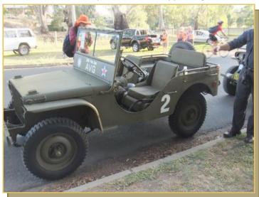
P-80 inch wheelbase. This is the 2nd prototype made by Ford which competed with the Willys MA and the Bantam BRC 40, to win the US Quartermaster's contact for a light reconnaissance vehicle.
