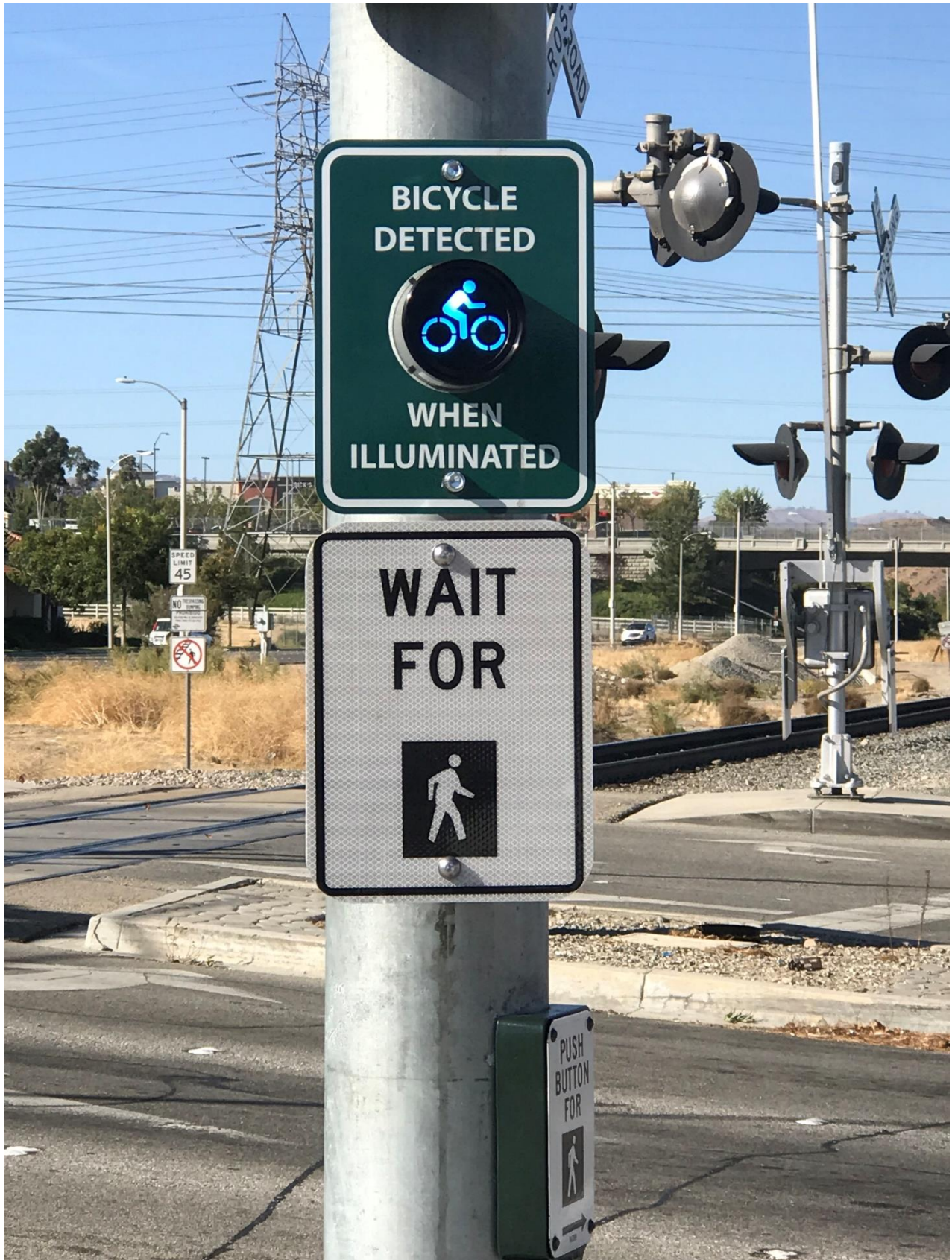
Bicycle indicator light informing the cyclist that they have been detected.
