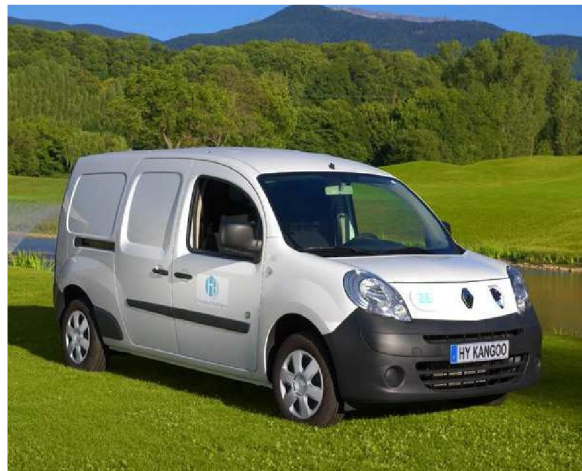
La Poste : 3 vehicles, Renault Kangoo ZE with Symbio Range Extender H2
