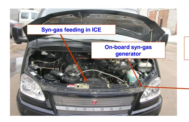
On-board converter with nanostructured catalysts
