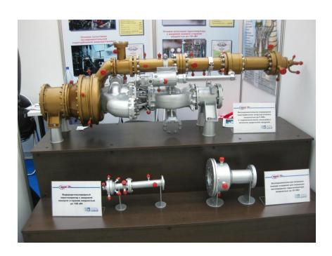
A model high temperature steam turbine unit with hydrogen-oxygen steam combustors of up to 5 MW capacity has been designed and tested by Joint Institute for High Temperatures and JSC "Chemical Automatics Design Bureau". Currently demonstration project with hydrogen-oxygen steam generator integrated in turbine units is being prepared.
