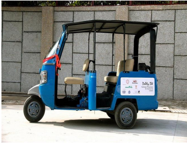
DELHY 3W, Hydrogen fuelled Passenger 3 Wheeler
