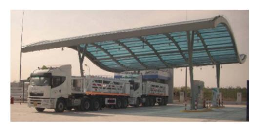
Developed by Shanghai Sunwise Energy System Co., two mobile HRS were put into operation on April 15.
