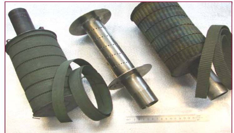
Tape catalyst reactor of the syngas capacity ca. 5 m 3 /hour
