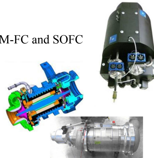
Automotive PEM compressor (18kW, >2.5bar)
