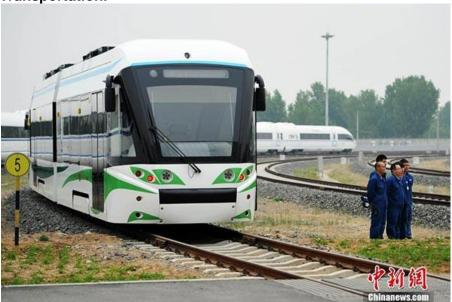
A hybrid tram powered by hydrogen cells and super-capacitors rolled off the assembly line in North China's Hebei province, April 27, 2016. According to Tangshan Railway Vehicle Co Ltd (TRC), the tram's major developer, this pollution-free tram can carry 336 passengers. A 15-minute hydrogen refill can power the vehicle for 40 kilometers at speeds as high as 70 km per hour.
