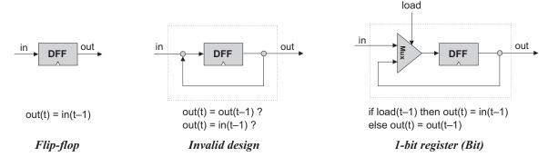
**Figure 3.1** From a DFF to a single-bit register. The small triangle represents the clock input. This icon is used to state that the marked chip, as well as the overall chip that encapsulates it, is time-dependent.
