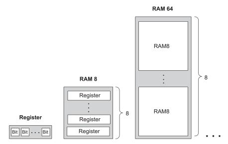
**Figure 3.6** Gradual construction of memory banks by recursive ascent. A *w*-bit register is an array of *w* binary cells, an 8-register RAM is an array of eight *w*-bit registers, a 64-register RAM is an array of eight RAM8 chips, and so on. Only three more similar construction steps are necessary to build a 16K RAM chip.
