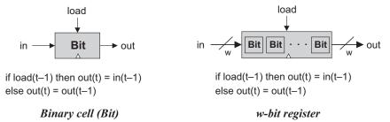
**Figure 3.2** From single-bit to multi-bit registers. A multi-bit register of width w can be constructed from an array of w 1-bit chips. The operating functions of both chips is exactly the same, except that the "=" assignments are single-bit and multi-bit, respectively.
