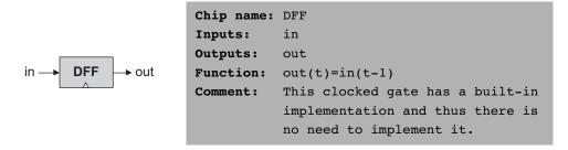
Like Nand gates, DFF gates enter our computer archtecture at a very low level. Specifically, all the sequential chips in the computer (registers, memory, and
