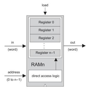
Figure 3.3 RAM chip (conceptual). The width and length of the RAM can vary.
