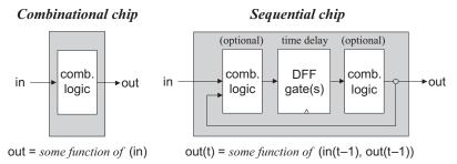
**Figure 3.4** Combinational versus sequential logic (in and out stand for one or more input and output variables). Sequential chips always consist of a layer of DFFs sandwiched between optional combinational logic layers.
