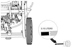
NOTICE: Pause to permit oil to settle. Wipe dipstick clean each time oil level is checked. DO NOT Overfill.
