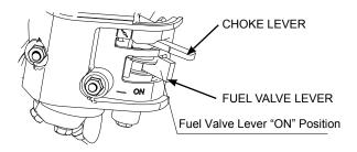
11. Move the choke lever to "Choke" position.
