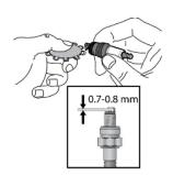
6. Install spark plug, tighten securely.
