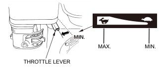
13. When starting engine, position yourself as recommended below and grasp starter grip handle and pull slowly until you feel some resistance. Then pull rapidly to start engine.
