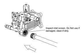
**IMPORTANT!** NEVER siphon standing water for the water supply. Use only cold water (less than 100 °F).
