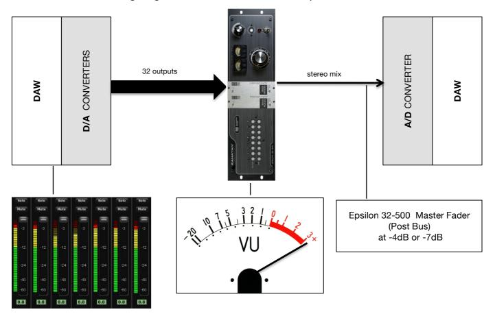
In a "saturated" mix the DAW output levels are "high". Inside our summing bus the signal levels are will be off the scale and the Epsilon 32-500 master fader requires attenuation. This is the same situation when using an analog console the master vumeters are off scale. The Epsilon requires that the master fader attenuate the output levels to send the mix to DAW or other analog gear.
