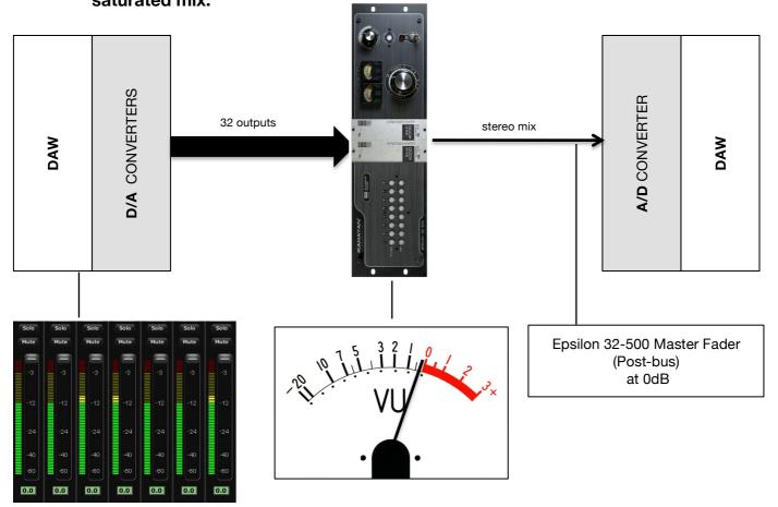
In a "clean" mix the DAW output levels are normal or "low". Inside our summing bus the signal levels are will be closet o 0VU=+4dBu and the Epsilon 32-500 master fader doesn't require attenuation, it's positionated at 0dB. **Remember:** the master fader is post-summing bus.
