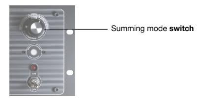
**1- 500 SERIES.** This first summing mode allows you to use 500 series modules thru the 2 space rackmounts that the Epsilon 32-500 has. You can use our 500 series modules or any 500 series preamps.
