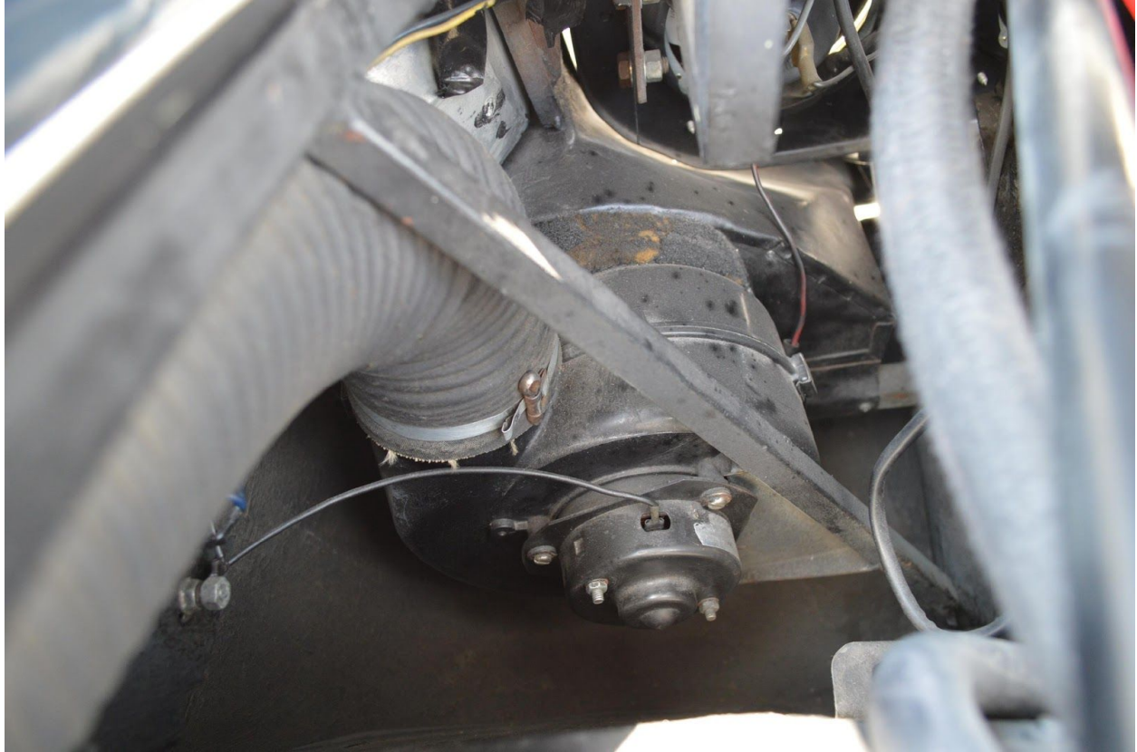
47. Untouched heater hose, clamps, motor. and wiring. Daytona Speciale. Image Dustin Wetmore
