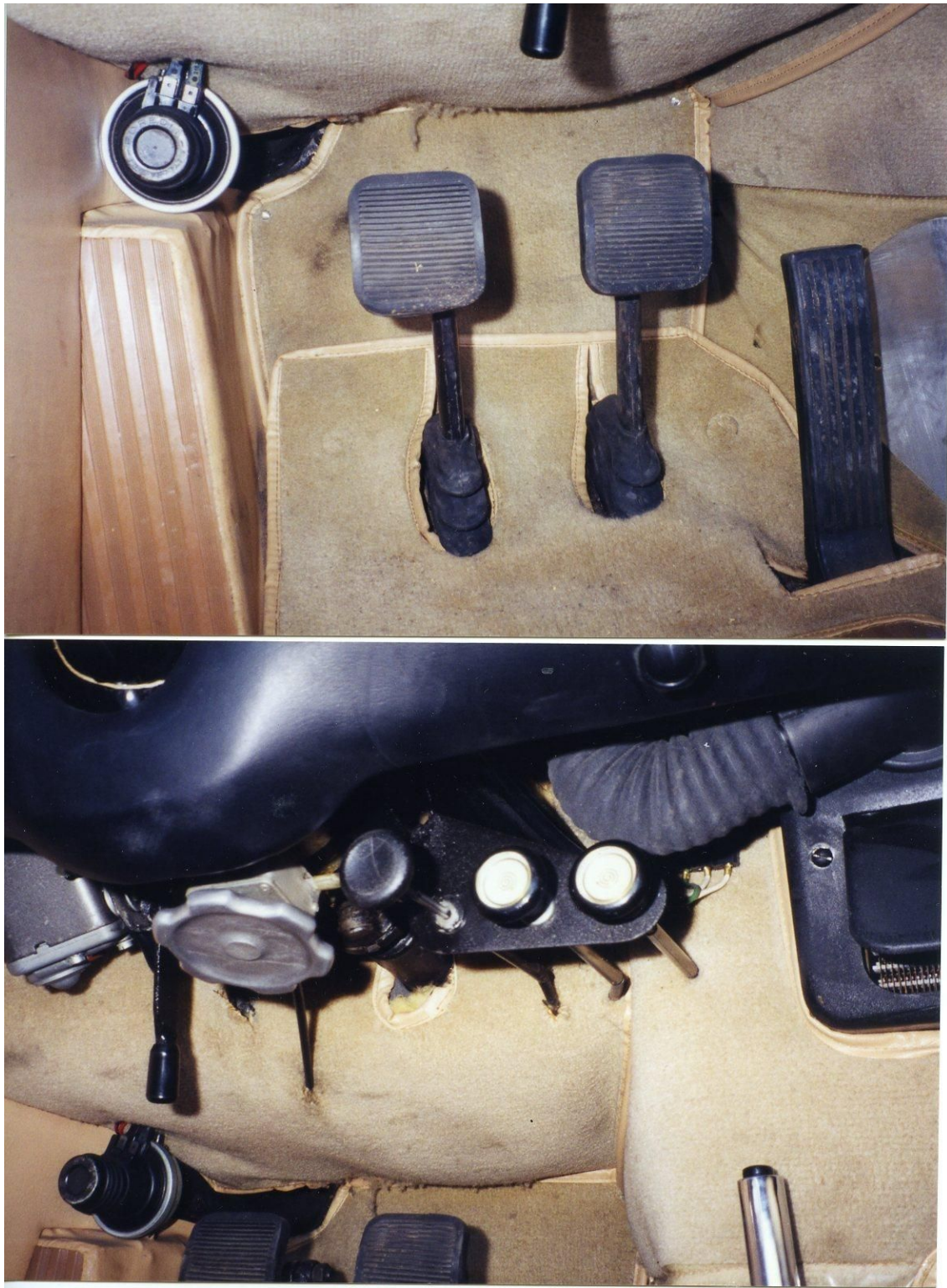
23. Rough fit, uneven stitching and untrimmed cut-outs reflect typical Scaglietti practice. 250 Lusso. Image David Carte
