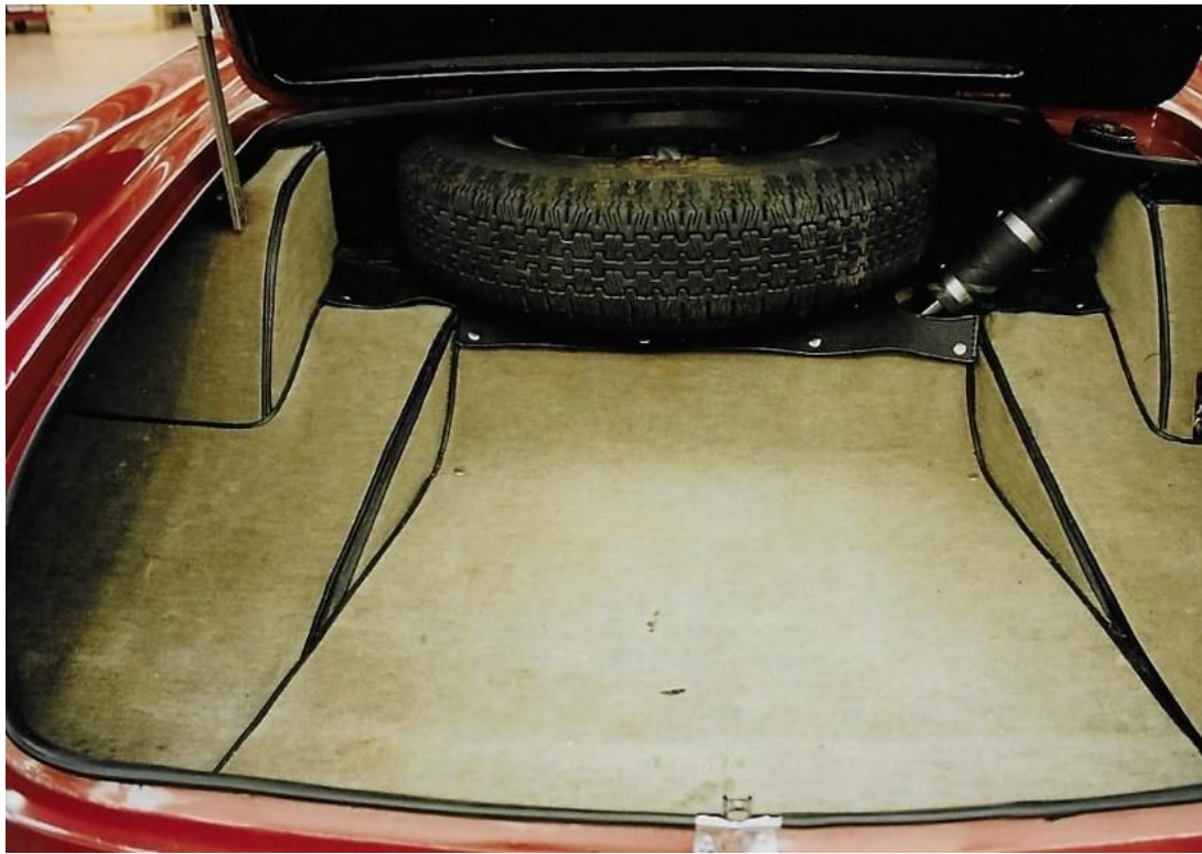
16. Original trunk and carpeting. Modern clamps and tire. Missing wiring block cover. 250 Cabriolet. Image David Carte
