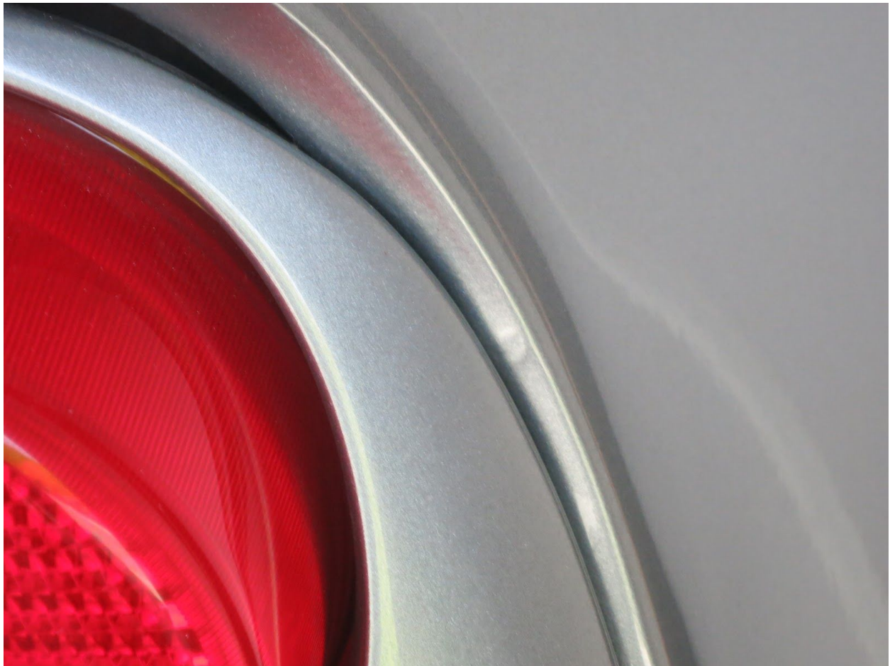
48. Typical factory paint blemish as delivered in unlikely to notice taillight area. Original 355. Image Donovan Leyden
