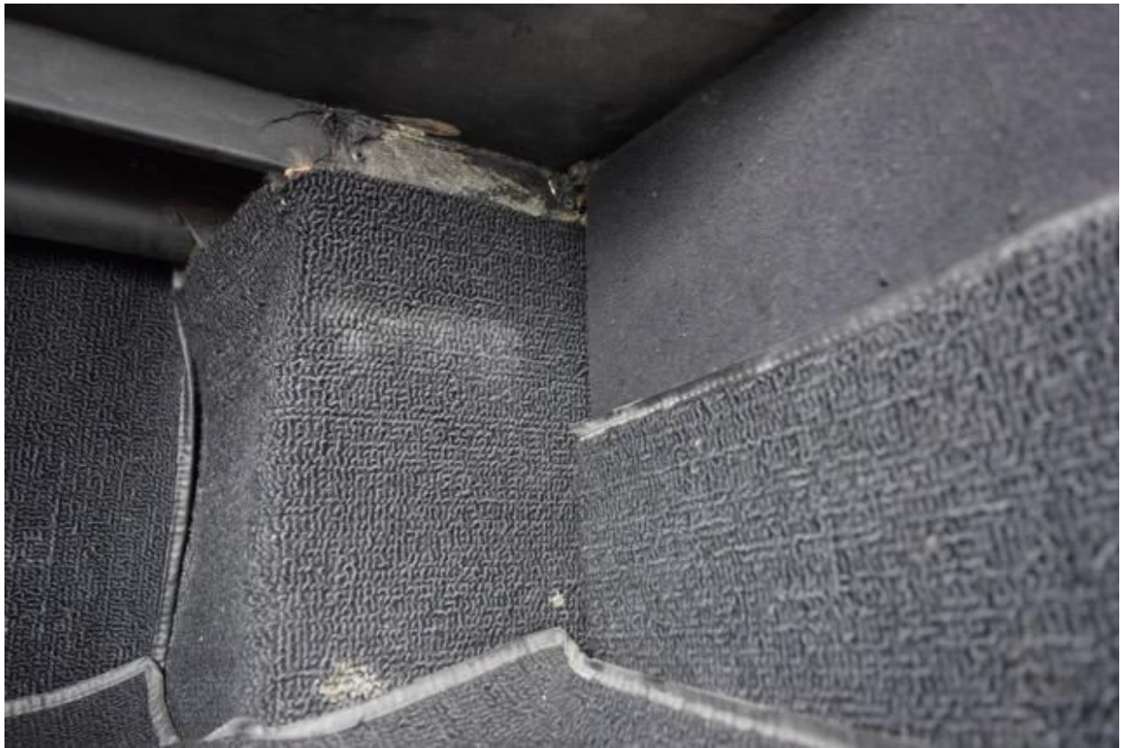
24. Trunk carpet, untrimmed as built with glue overlap on frame. 246 Dino. Image Marco Hartner.
