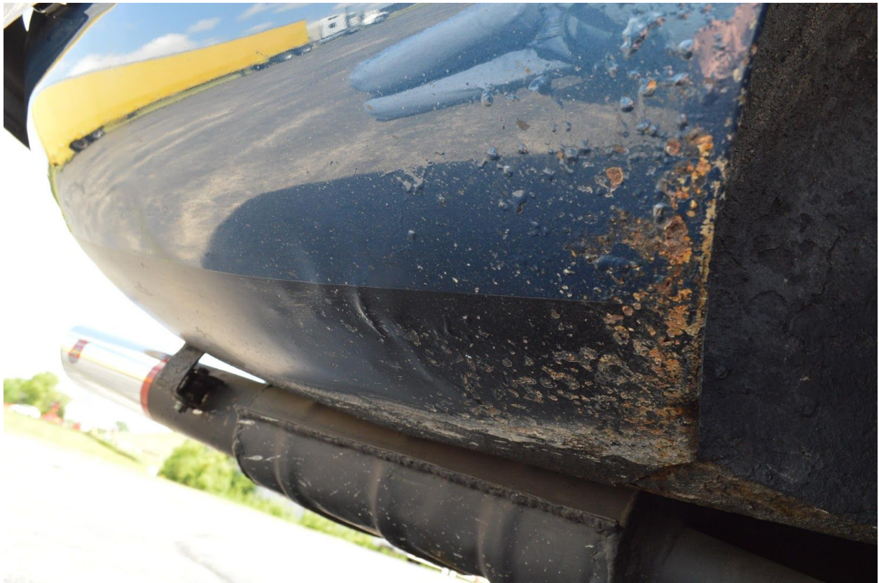
43. Original Daytona Speciale resonator with limited repair (welded cap). Owner resisted temptation to repaint despite some surface rust. Daytona Speciale. Image Dustin Wetmore
