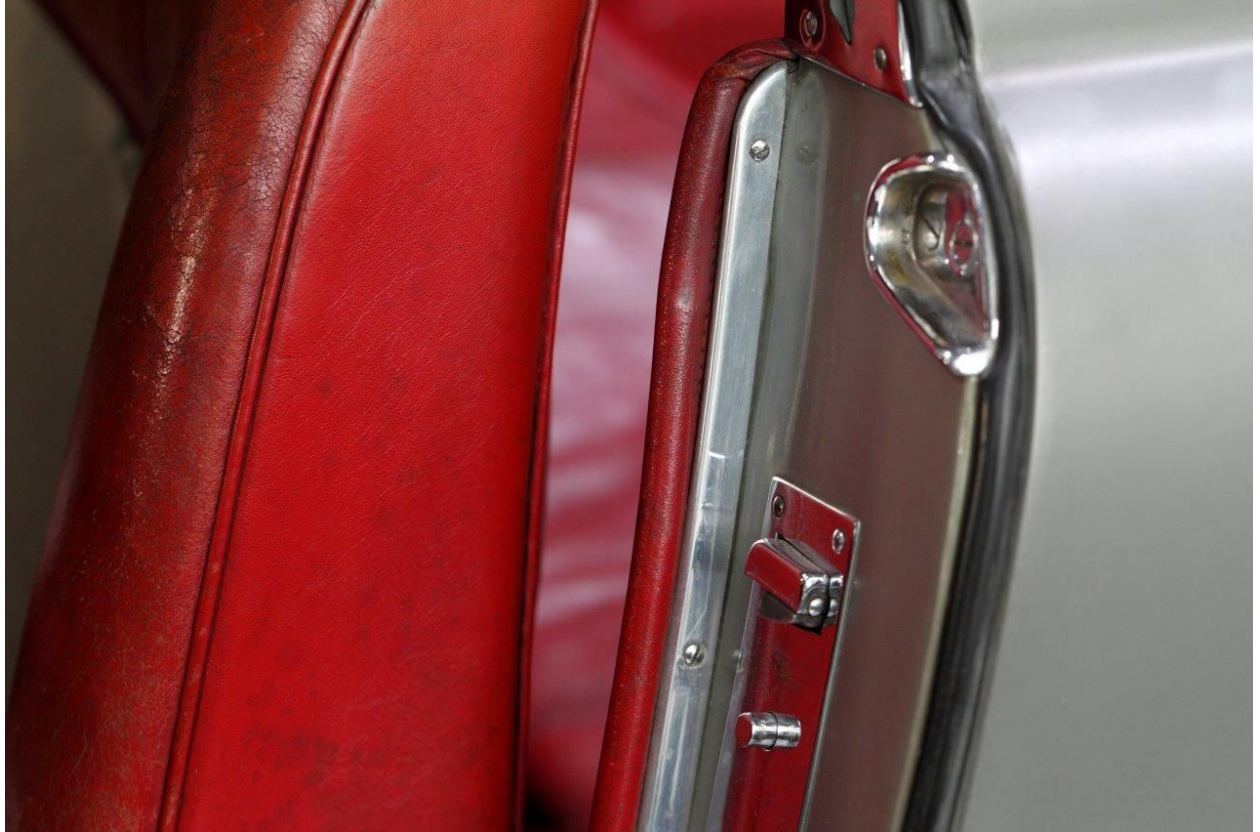
26. Unrestored interior with original door jamb chrome and rubber seal. 250 Europa. Image David Carte
