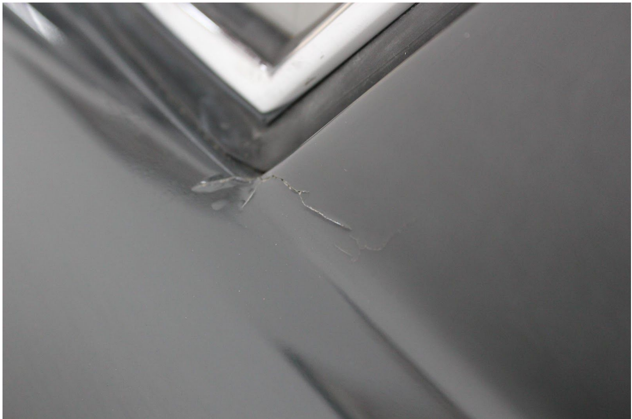
6. Typical cracking in older lacquer paint. 250 Coupe. David Eichenbaum
