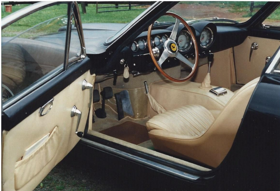
35. Original interior, puckered door pocket and console and plastic scuff guard. 250 Lusso. Image Greg Jones
