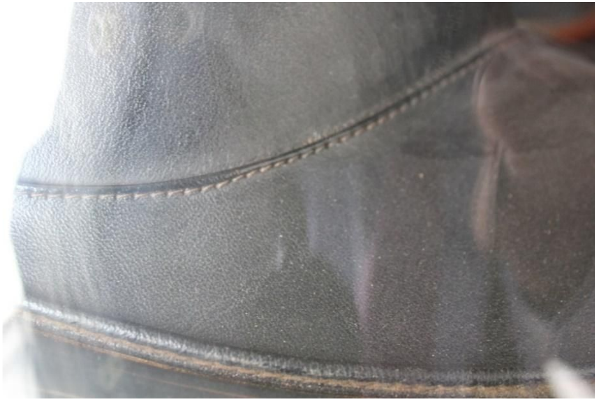
5. Original seats show grain, piping, stitching and workmanship. 250 Coupe. Image David Eichenbaum
