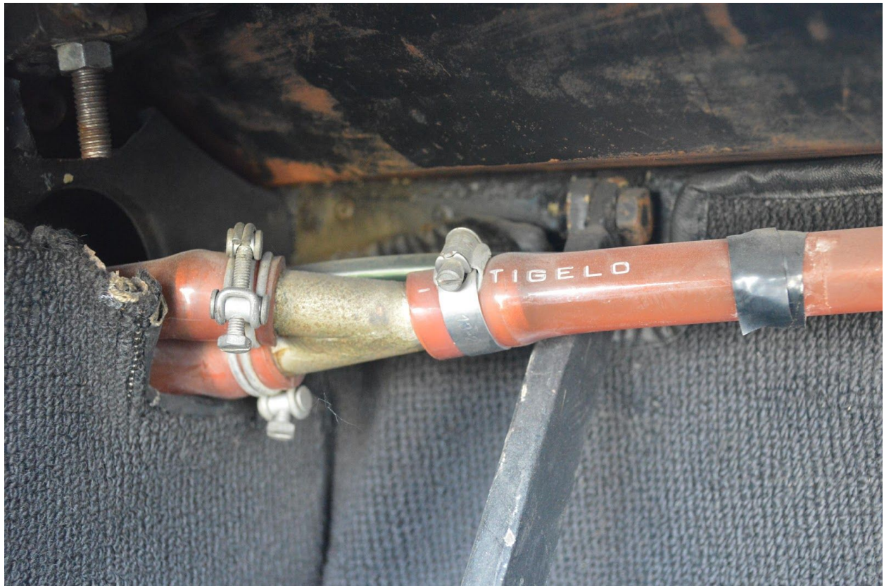
45. Unmolested original trunk, fuel vapor hose and clamps. Daytona Speciale. Image Dustin Wetmore
