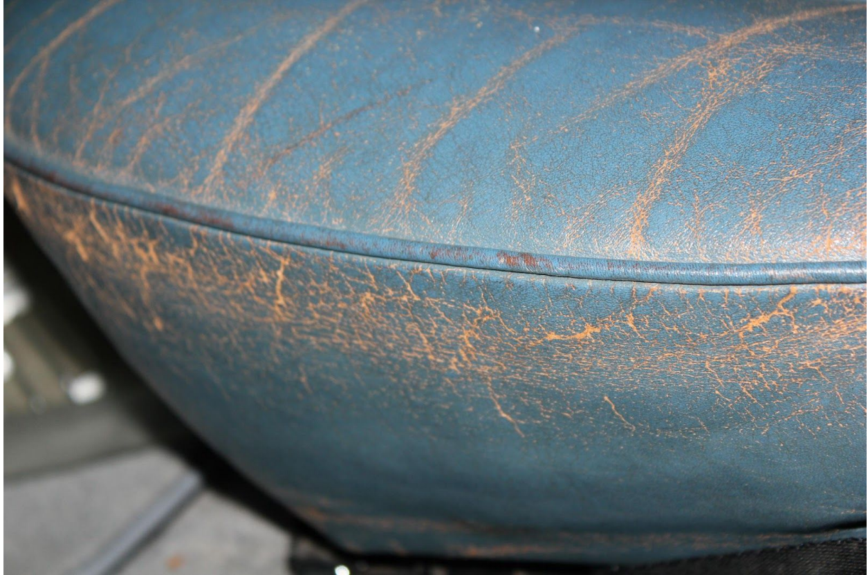
4. Detail of original leather dye and piping with original material underneath. 250 Coupe. Image David Eichenbaum
