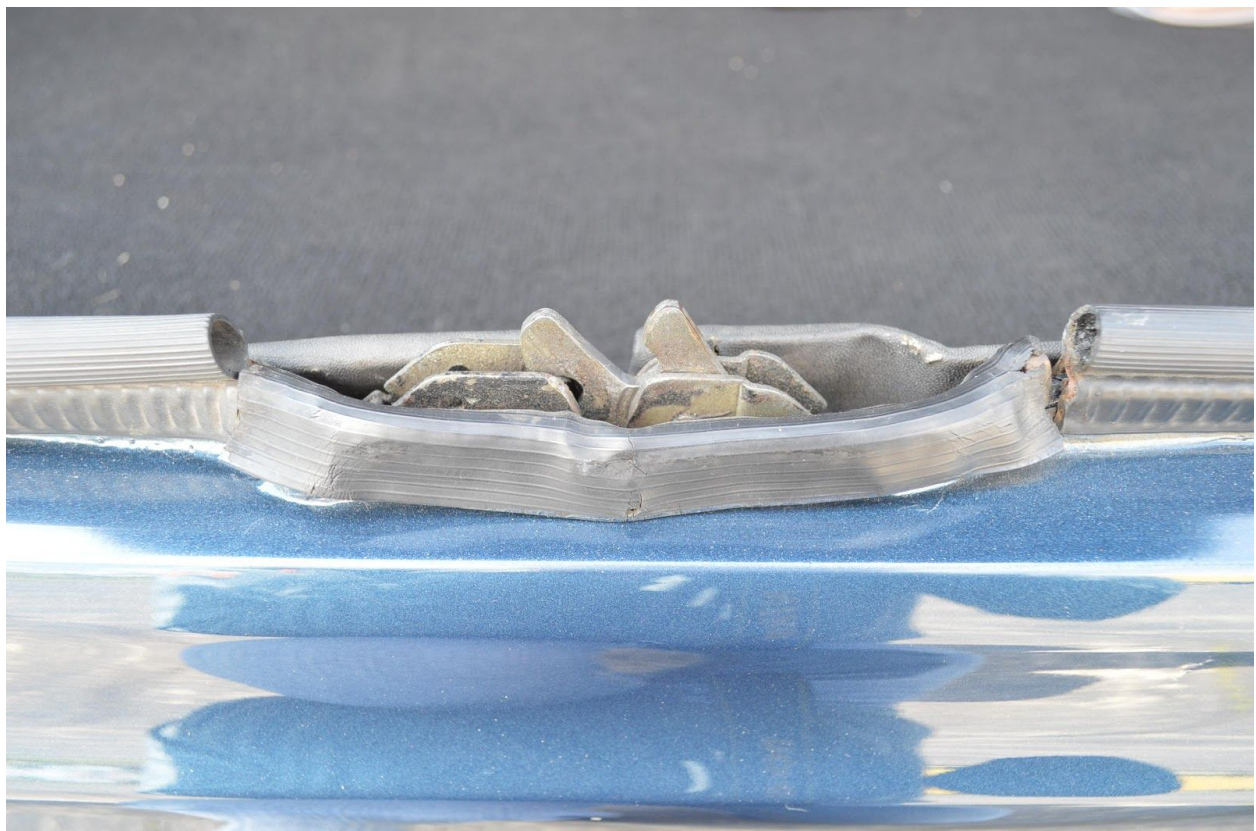
45. Unmolested original trunk, fuel vapor hose and clamps. Daytona Speciale. Image Dustin Wetmore
