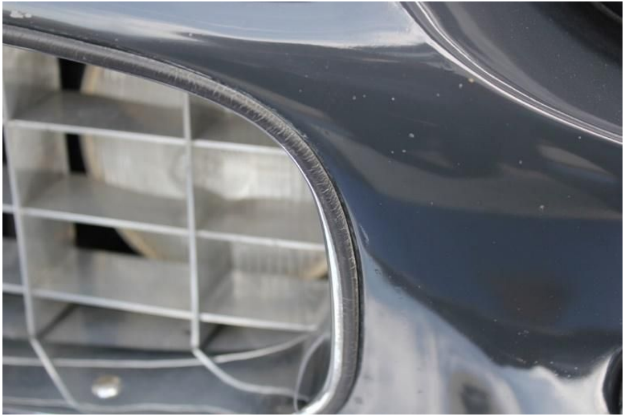
7. Molding showing wear still performs original function. 250 Coupe. Image David Eichenbaum
