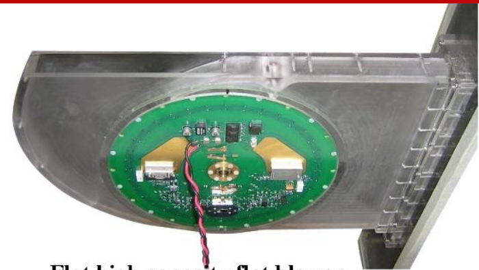
Flat high capacity flat blower THK 22 mm V = 140 cfm
