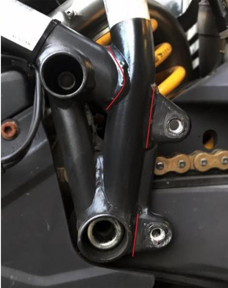
**Figure 2.** Areas of potentially high welds
