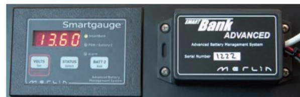
difference is the sensor circuitry and the relay/s are separate modules, allowing the latter to be mounted close to the batteries, thus shortening heavy-duty cable runs. On the three-bank model a second relay makes in conjunction with the first, bringing a third battery into the charging circuit. As the sensing is only done on the battery one terminal and both relays
