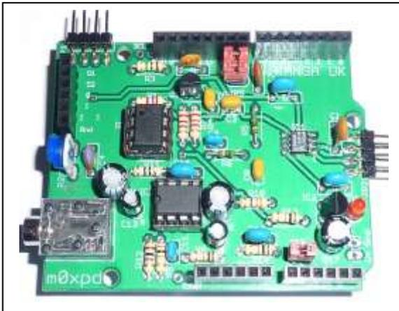
The Kanga / mØxpd Arduino Rx Shield is a simple Direct Conversion receiver sub-system for the HF bands.
