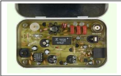
The FOXX-3 by Derek Alexander G4GVM was published in the spring 1999 issue of SPRAT. While based on the original FOXX, it had a few refinements to make operation easier: Automatic transmit/receive change over (semi-break-in), sidetone and built in harmonic filter. Derek has kindly given Kanga Products permission to produce the FOXX-3 in kit form.
