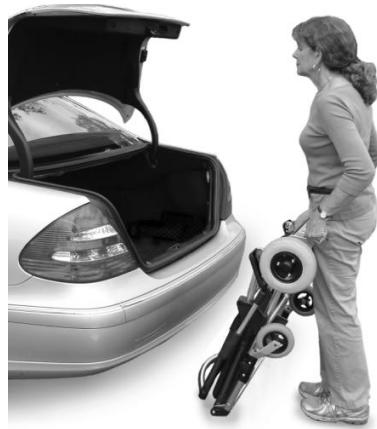
Grab the Anti-Tip Wheels and lift the rear of the Zinger so that it leans against your upper thighs as shown.
