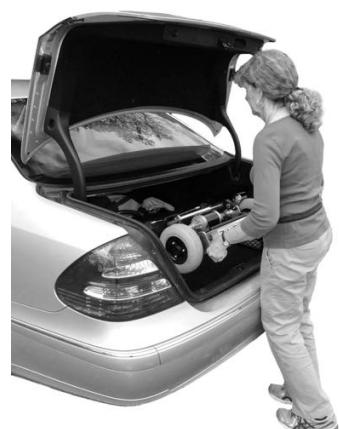
Finally, slide the Zinger into the trunk and set it down by holding the Anti-Tip Wheels.
