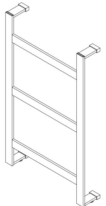
TEST PRESSURE: 6 BAR MAX WORKING PRESSURE 3 BAR MAX WORKING TEMPERATURE: 100°C HEAT OUTPUT DETERMINED IN ACCORDANCE WITH EN 442 ZINGO SULTAN WALL MOUNTED TOWEL RAIL 1000 x 600mm - HYDRONIC
