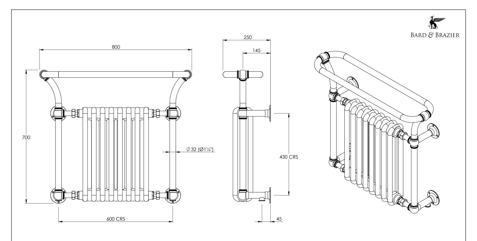
BTU/HR AT DELTA 60: TEST PRESSURE: 3319 CONNECTIONS: FI 1/2" BSP MAX WORKING PRESSURE MAX WORKING TEMPERATURE: HEAT OUTPUT DETERMINED IN ACCORDANCE WITH EN 442 BARD & BRAZIER LIMITED T: +44 (0) 121 270 2222 TITLE: MARSTON ROAD E: INFO@BARDBRAZIER.CO.UK WOLVERHAMPTON
