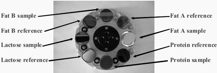
**Each filter selected a different range of mid-IR light wavelengths. The filter wheel had to rotate and stop in the light beam to take a reading with each filter for each sample.**
