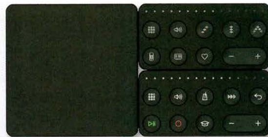
Fig. 3. Loop Block and Live Block attach magnetically to the Lightpad Block.
