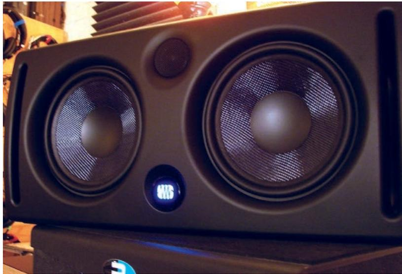
The Eris line (including the smaller E44) employs a D'Appolito arrangement—or MTM, midwoofer/tweeter/midwoofer—with a pair of identical 6.5-inch Kevlar fiber woofers sharing the same frequency range.
