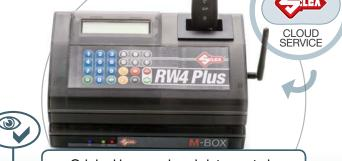
Original key read and data sent via cloud to Silca for processing. Maximum estimated time to completion indicated in RW4Plus display.
