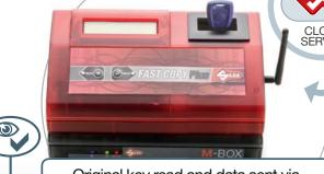
Original key read and data sent via cloud to Silca for processing. Maximum estimated time to completion indicated in Fast Copy Plus display.
