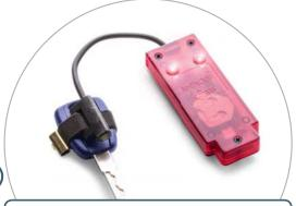
Data detection. Wrap the M-Snoop around the customer key and turn the key in the car ignition 3 times. M-Snoop LEDs illuminate to confirm successful sniffing.
