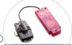
Data detection. Wrap the M-Snoop around the customer key and turn the key in the car ignition 3 times. M-Snoop LEDs illuminate to confirm successful sniffing.
