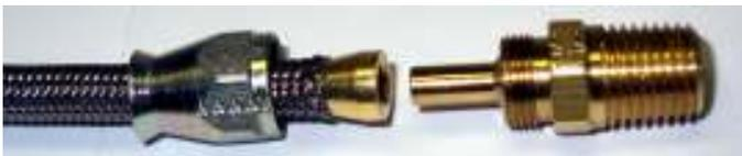
Finally, take the last part and insert the brass tube into the hose. Be careful to make sure the small tapered part is still sealed over the Teflon. Screw the two fittings together, making sure the bottom fitting does not dislodge the small tapered piece. Once you are done it looks like below. Try to pull apart, it should not come apart.
