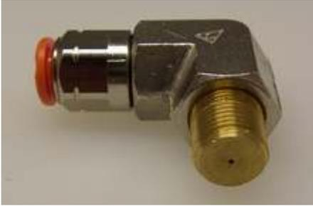
The injector is 1/8<sup>th</sup> NPT. If you have an intercooler we recommend placing between the intercooler and throttling body. Never place prior to the turbo. If you have a roots style supercharger its acceptable to place prior. Drill your intake with 11/32-drill bit and then tap with 1/8<sup>th</sup> NPT (27 threads per inch). The injector will then screw in. If you run multiple injectors space the injectors a minimum of 6 inches apart for best performance.
