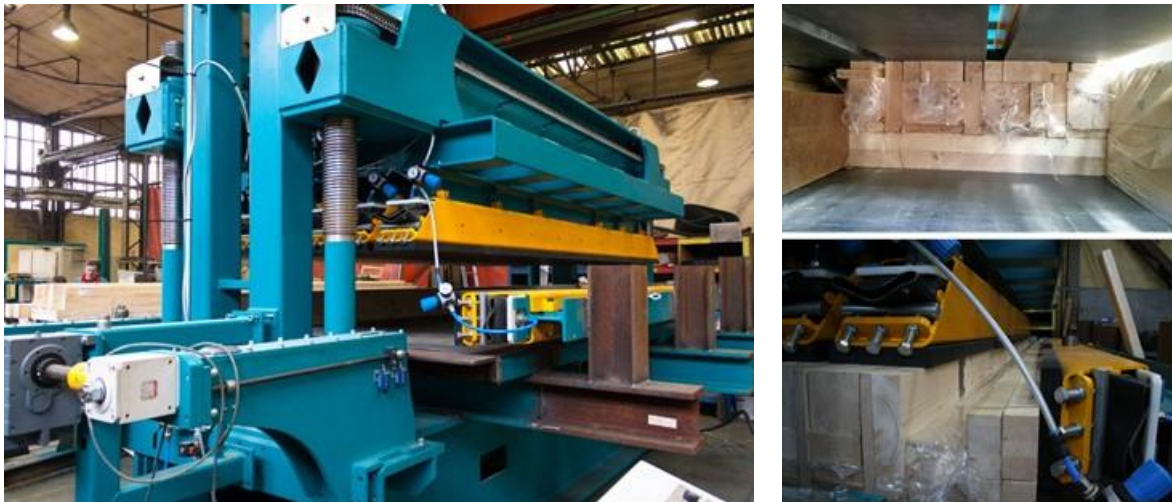
Figure 6: Large specimen production; vertical pressing over dummy elements and side pressing
