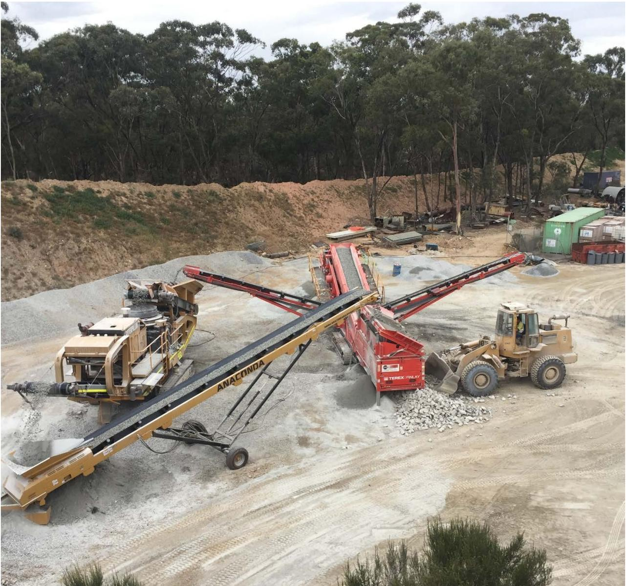
**Figure 2: Secondary ‘Cone’ Crusher, screen and grizzly, Porcupine Flat Processing Facility**
