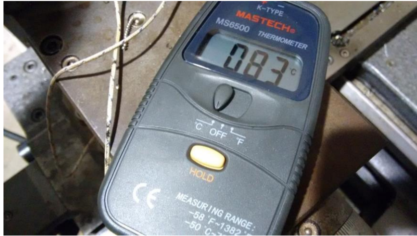
Figure 4.5: Temperature reading on digital thermometer while machining AISI 1045 with heat pipe installed in carbide insert
