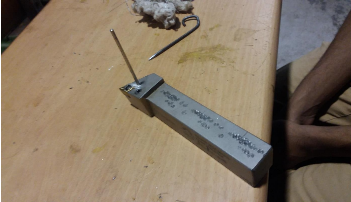
Figure 4.2: Carbide insert tool with heat pipe
