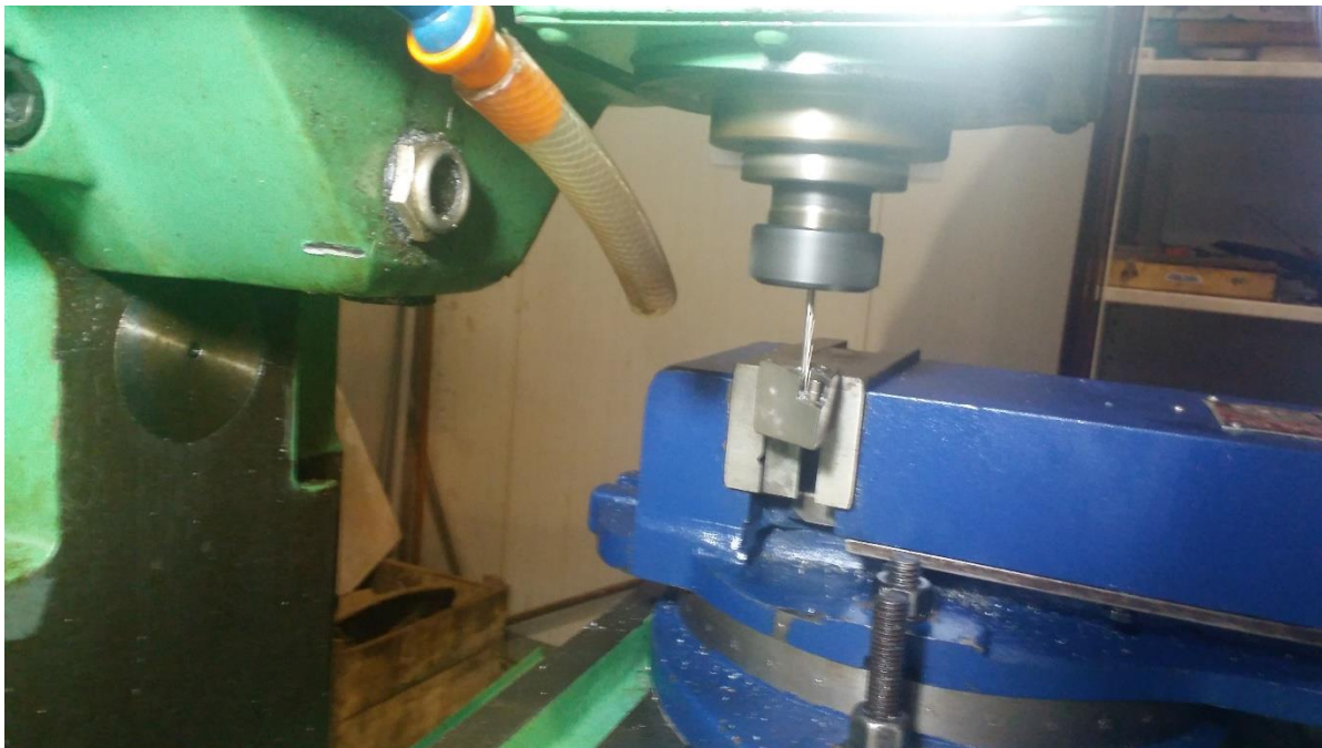
Figure 4.1 : Drilling a hole in the tool holder for the installation of heat pipe
