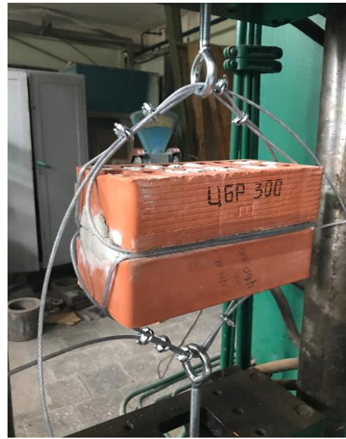
Fig. 5. Determination of the The compressive strength (a) and adhesive strength (b) of the brick masonry using a modified building mortar
