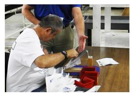
One of the accommodations we made allows participants with limited hand use to assemble and package hardware. The fixture holds the bag open while participants sort and slide required components into the package.
