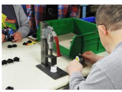
tomer specifications with a high degree of consistency. The fixture allows the perfect assembly of terminal covers each and every time.
