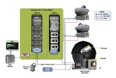
The diagram to the left depicts a HALO System Ground Node which can be situated on the roof or adjacent to a Customer PoP or Telco Shelter Location.
