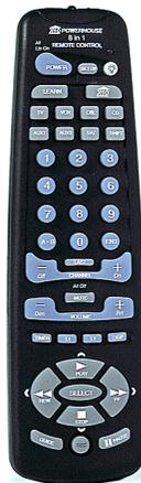
This device has a normal infrared output, to control infrared appliances such as TV, video, stereo and some air conditioners. But it also has an RF output; in combination with a Transceiver Module (a device that plugs into a power point and converts RF signals to X-10) this remote can control any facility or appliance that is powered through your wiring, such as lights, fans, heaters. It can also be set up to control doors, curtains and other specialised products.
