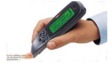
From the same manufacturer, we have a pen that reads text aloud to you. Just roll this pen across typed text and it will read the text to you. It can read a single word or whole line. The text is also displayed in large characters on the pen's screen. The pen has a dictionary of 200000 words and it can read the definition to you. You can adjust the speech volume, speed and pitch.
