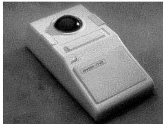
This trackball has integrated hand support and a middle button that can be programmed easily as Click, Double-Click or Click & Drag. It has a built in scroll feature and extremely light ball movement force. Stainless steel shafts and bearings should ensure a trouble-free life.
