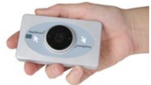
The HeadMouse Extreme is powered by the USB or PS/2 bus, with low (approximately 1-watt) power consumption. The small (3.7x 2.2x 0.5 inch) case and flexible mounting options give the user a range of options. The cost of the HeadMouse Extreme is US\$995, probably landing here for an estimated price of A\$1400. It will be available through Ability.
