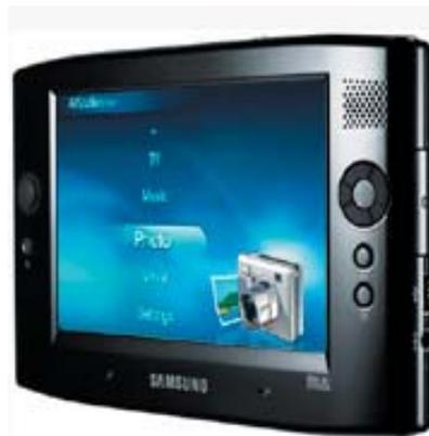
Size is 229 x 140 x 25mm. It weighs 770g. Battery life is 3 hours, or up to 6 hours with the optional 6 cell battery.
