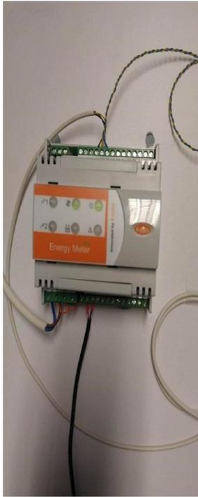
Figure 3b Picture of the 3 phase power meter
