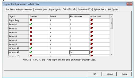
Note: A different output number can be selected from the signal list. 'Output #2' is turned on by the G-code command 'M11P2' and turned off by 'M10P2' If a different output number is required, change the '2' in the code snippet to the required number when creating the rules in SheetCAM. For details, see section 3.2.
