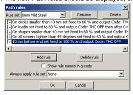
12. When creating a Jet cutting operation in SheetCAM, select the required rule from the 'Path rules' drop-down. This will use improved cut techniques and turn the height control on and off when required. If the rules are working correctly, the M10P2 and M11P2 commands should appear in the G-code file.
