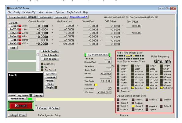
To verify the anti-dive signal, go to the output signals configuration screen and click on 'Active Low' to change the state of the signal. If anti-dive is enabled on the AVHC10, this will make the two blue LEDs on the AVHC10 light together to show anti-dive is activated.
