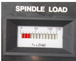
1. You can calculate the duty cycle for a part (= Cutting time / total cycle time) and use the S6 rating to determine how much you can load the spindle.
