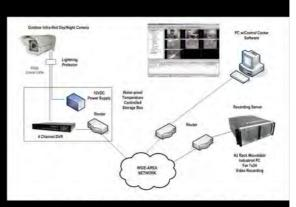
Main Components of the system : Day/night Indoor/Outdoor Infra-red color Camera; Digital Video Recorder (DVR); Desktop computer; Control Center software; Routers etc.
