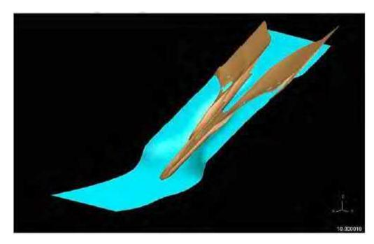
Debris flow simulation using conventional Lagrangian meshing method
