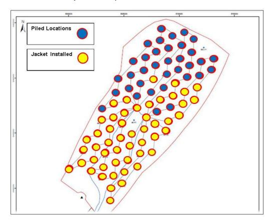
Fig. 2 Pile installation completed at 86 Locations
