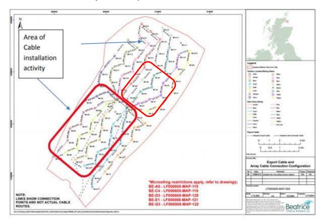
Fig. 5 Inter Array Cable Installation work location
