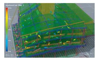
For example, the whole basement withstood collapse entirely and the midway shear core that contained lifts and stairways tilted eastwards. Thereby, the upper-floor slabs formed voids at the transition to the lift shaft. Reports by rescue personnel that arrived at the site short after the earthquake show that some survivors were indeed found in the collapsed building in similar cavities.
