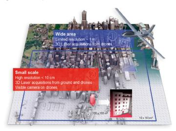
High-resolution and high-quality digital elevation/surface models (DEM/DSM) are fused from these two approaches (laser imagery and high-resolution images).
