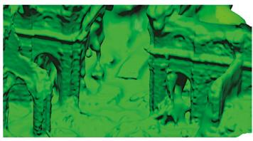
The similarity between the laser and image-based 3D model of a collapsed building and the collapse simulation model of the same building opens the opportunity to infer the location of several building elements inside a collapsed building.
