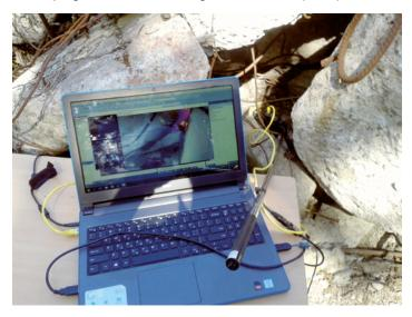
The main challenges of the LWIR development are the operational environment, which may be characterised by smoke, dust, rubble and extremely narrow spaces, as well as the very low resolution caused by the continuously moving LWIR camera.
