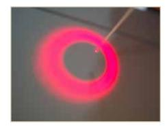
**Figure 4.** Radial Tip Fiber, 360° Dispersion Pattern
