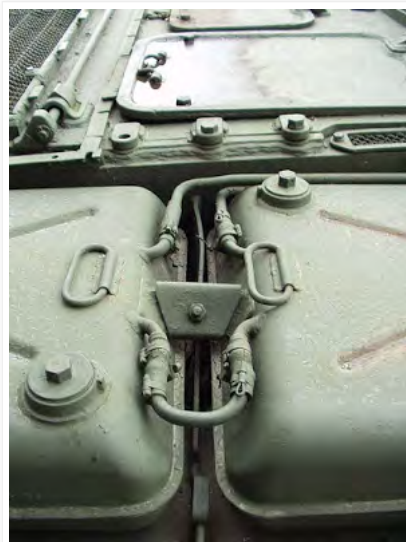
Here you can see how the fuel tanks are connected
