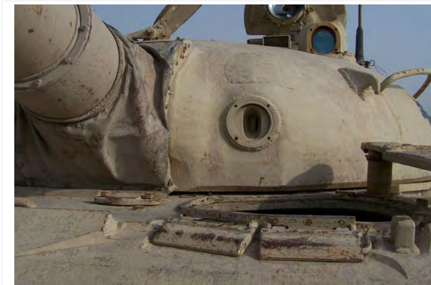
Telescopic sight aperture port, with nuclear attack seal in place
