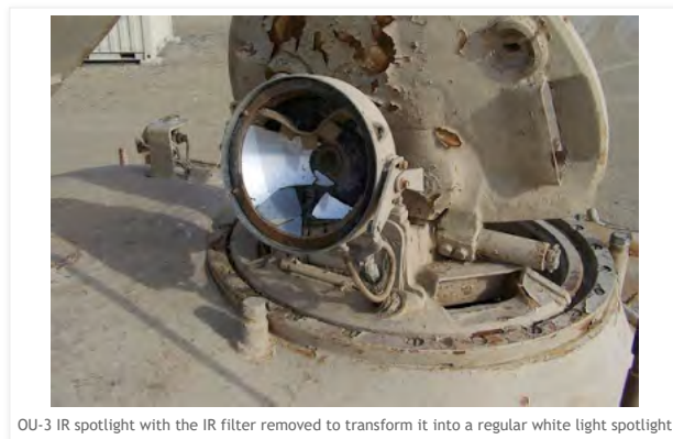
OU-3 IR spotlight with the IR filter removed to transform it into a regular white light spotlight
