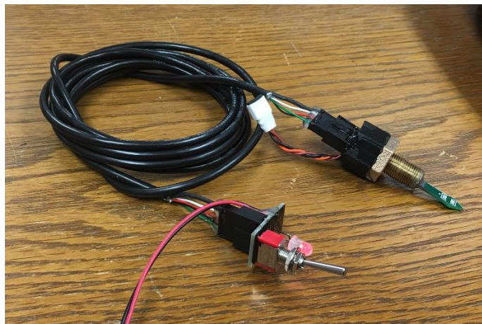
1: Bingo Fuel Detector with harness and switch / LED assembly
